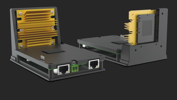
The PRM2141X development kit (DVK) is a cutting-edge solution designed for industrial and telecommunications markets that require high-speed wireless connectivity. The kit is built around the 60GHz wireless technology, which offers incredibly fast and reliable data transmission rates of up to 2.5Gbit/s, making it an ideal choice for use cases such as wireless backhaul, video streaming, and other bandwidth-intensive applications.
