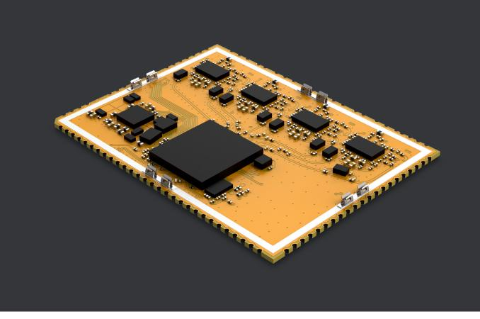
Pineapple is an 802.11ax Wi-Fi 6 and Wi-Fi 6E radio module for ultra-high speed enterprise connectivity. It is based on Qualcomm QCN9074 chipset for 2.4/5/6 GHz IEEE802.11ax/ac/n/g/b/ax applications. New radio can perform access point and station functionality with 4x4 MIMO (4 spatial streams). Pineapple is a wireless LAN radio with native 160 MHz support.
